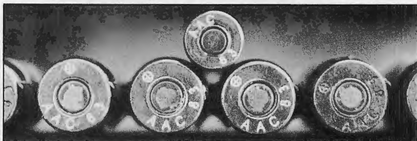
5.56x45mm NATO cartridge with counterfeit 'AAC 83' headstamp on top of linked belt of 7.62x51mm ammunition with similar counterfeit headstamp that includes the NATO cross in circle.
